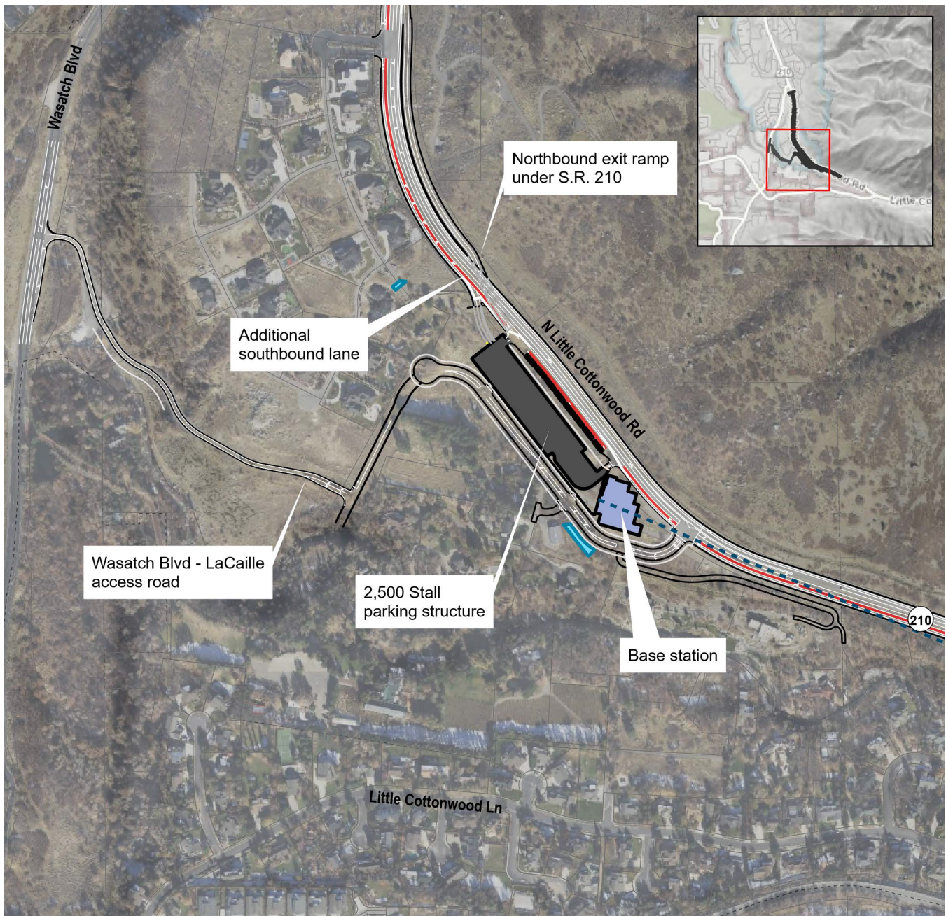
Figure 2.6-29. Gondola Alternative B – Base Station Layout South
