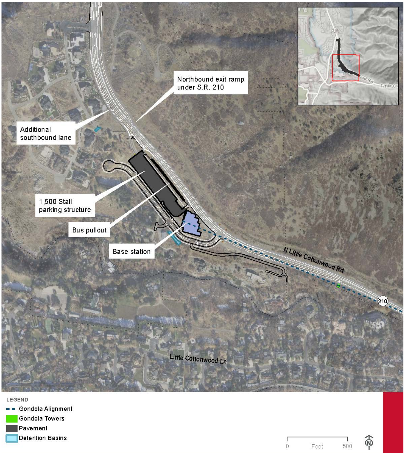
Figure 2.6-27. Gondola Alternative B – Base Station Layout South
