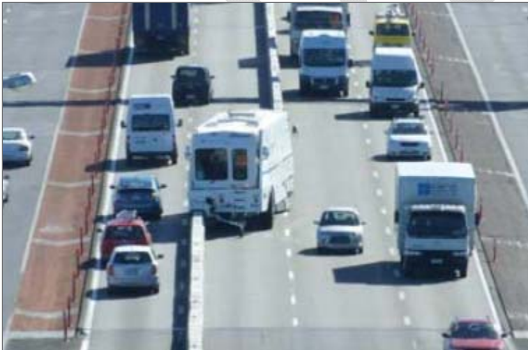
Figure 2-1. Moveable Barrier and Transfer Machine
