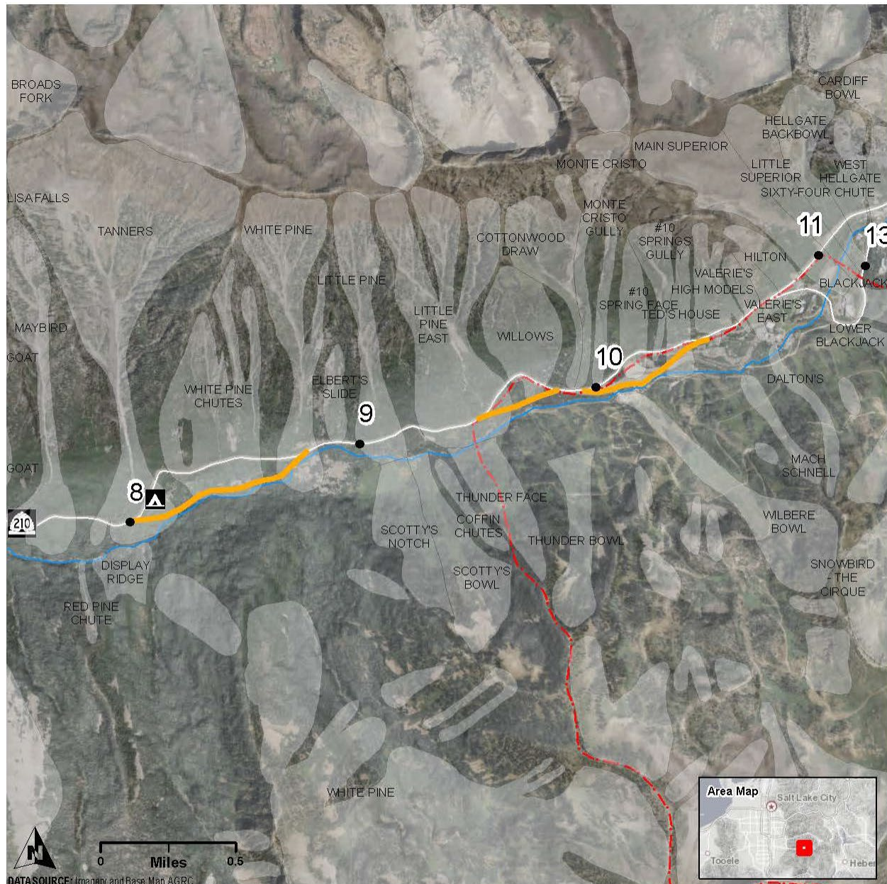
Figure 3-3. S.R. 210 Realignment for Avalanche Mitigation
