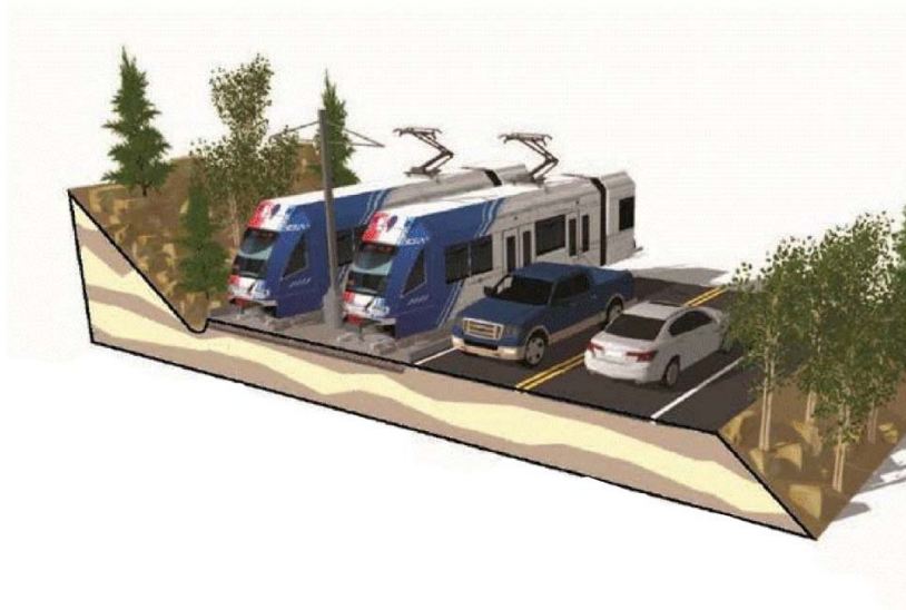
Figure 2. Conceptual Cross-section for a Cog Rail Line along Little Cottonwood Canyon Road
