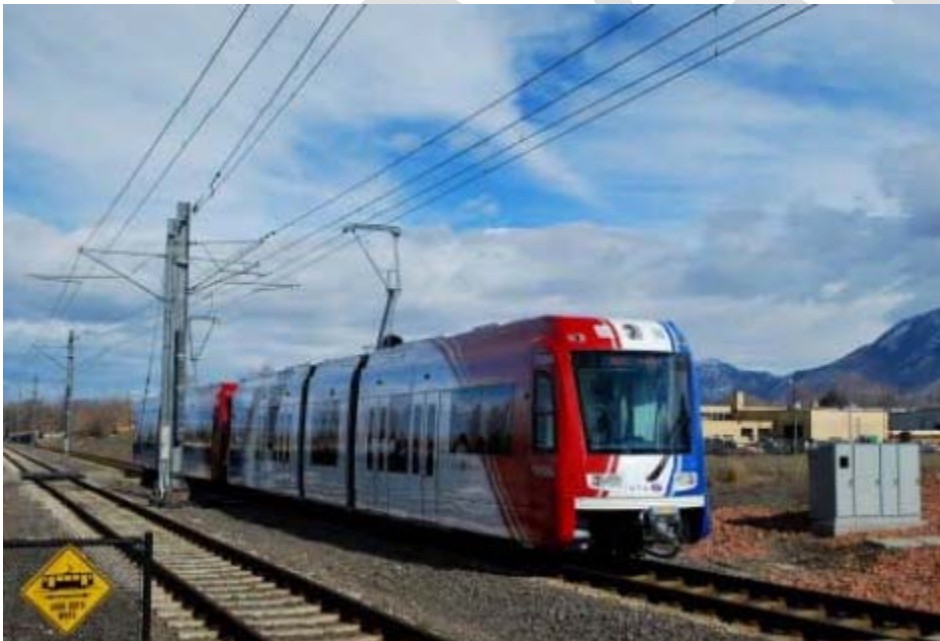
Figure 5. Example OCS and Pantograph
