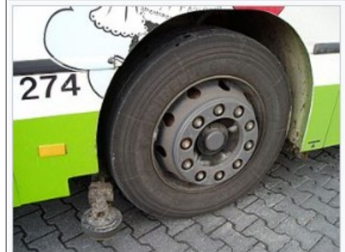
The kerb guide wheel of a guided bus in Mannheim, Germany
