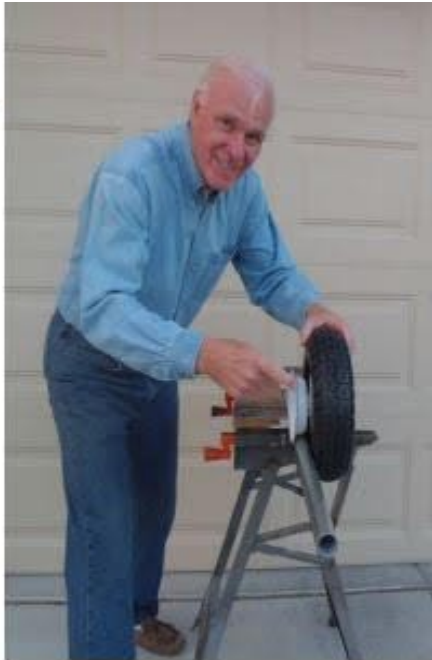
Dave Brough with a scale model of his Ezekiel 'wheel in a wheel' invention. It lets cars run both on pavement and on railway tracks
