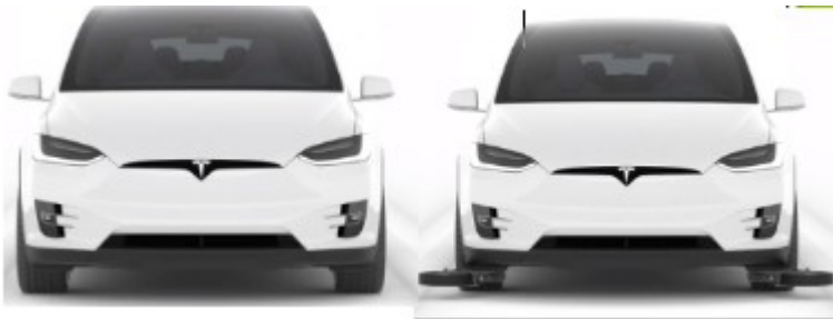
Boring Company's use of retractable 'kerb' guide wheels
